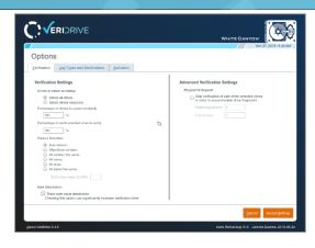
'Pattern Selection' allows you to select the expected pattern that VeriDrive will look for during the verification step. By default, the 'Auto-detect' option will detect the pattern based on the first few sectors of the drive and verify based on that.
