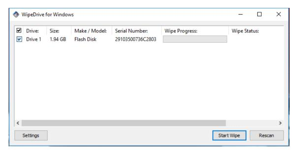
This is the main interface when using WipeDrive for Windows. Connected hard drives not containing Windows operating systems are listed along with other available information such as Size, Make/Model, and Serial Number (if available). After starting the wiping process the Wipe Progress bar will progress as the hard drive is erased. To begin erasing the hard drive(s), be sure only the drives you want to erase are checked and click "Start Wipe."
